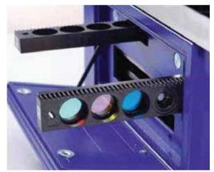
Due to their high transmission characteristics - which can be up to 25-fold that of monochromators - technologies like Time-Resolved Fluorescence (TRF) can be measured more efficiently with filters. In addition filters are available with wide bandwidths making them the ideal choice for fluorophores with wide spectra and for all luminescence based assays requiring the use of filters.
