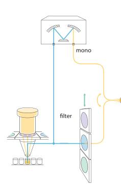
Flexibility in wavelength selection for any current and future assay requirements is best met by the ATL-MR 942S double-monochromator with high transmission and best blocking properties for absorbance and fluorescence excitation. Use the benefits of complete absorbance and excitation spectral scans to measure wavelength shifts due to e.g. changes in pH or polarity on the chromophore's properties.
