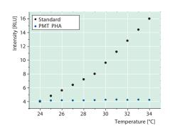
Noise Free Fluorescence Read-out with Pulse Height Analysis (PHA): The patent pending pulse-height-analysis detection mode operates almost background-free (dark count rate reduced by factor of 100). Temperature effects are significantly reduced and even at elevated temperatures, often required for cell-based assays, the dark count rate increases only marginally.
